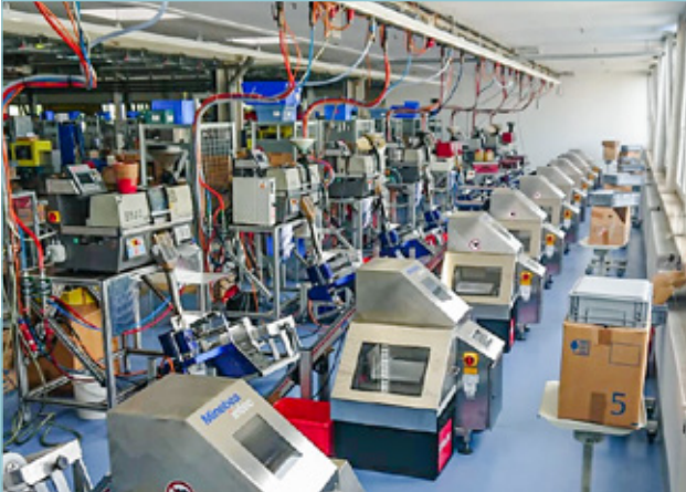
Thanks to specially developed covers, the weighing process is not affected by drafts
