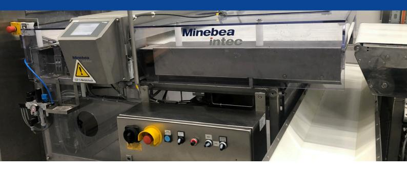
The chocolate manufacturer Weinrich wanted to integrate a metal detector into its existing production line. Alongside the limited space, the inspection solution also had to be able to cope with the product effect of chocolate and reliably detect foreign objects in the different varieties.
